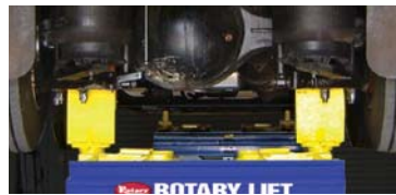
Example of adjustment range and rotated adapters with an off-set transaxle.
